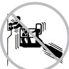
Do not replace items critical to machine stability with items of different weight or specification.
